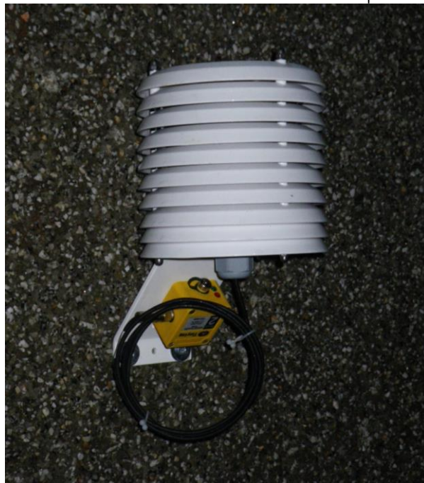
Figure 1: Example of a wall-mounted Stevenson screen for temperature and RH sensors
